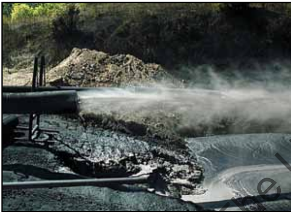
Figure 6.1. Gas and liquid exit the blowout line on a UBD rig. What occurs at the blowout line is not necessarily an indication of what is occurring downhole.
