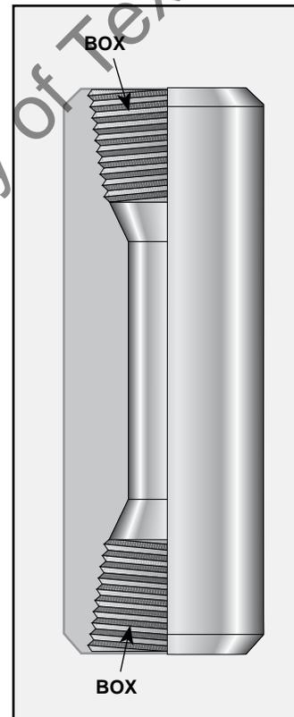
Figure 45. A bit sub; drawing shows a quarter-section taken out to show box threads inside the sub.
