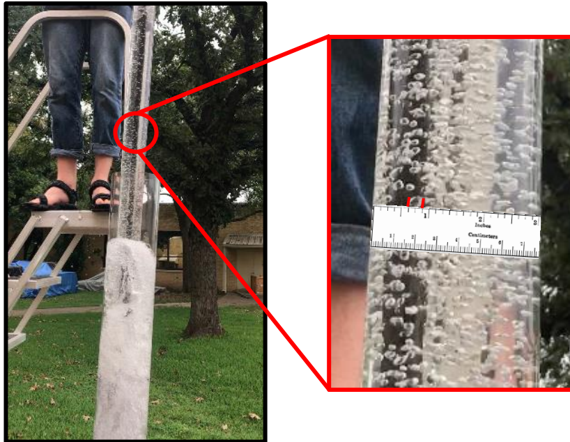
Figure 18 - Bubbles no larger than 0.25 inches inside pump
